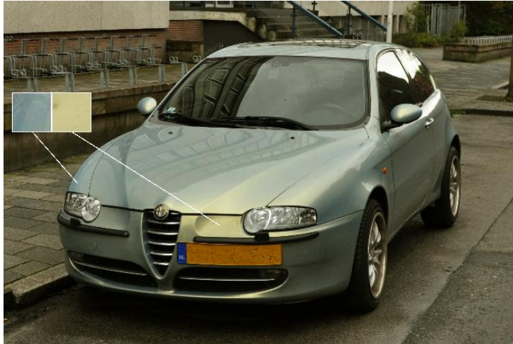
Figure 2. A car painted with pearl varnish. The different combinations of direction of light incident and direction of observation with respect to the metal surface can result to observation of complementary colours, like blue and yellow in this case.
